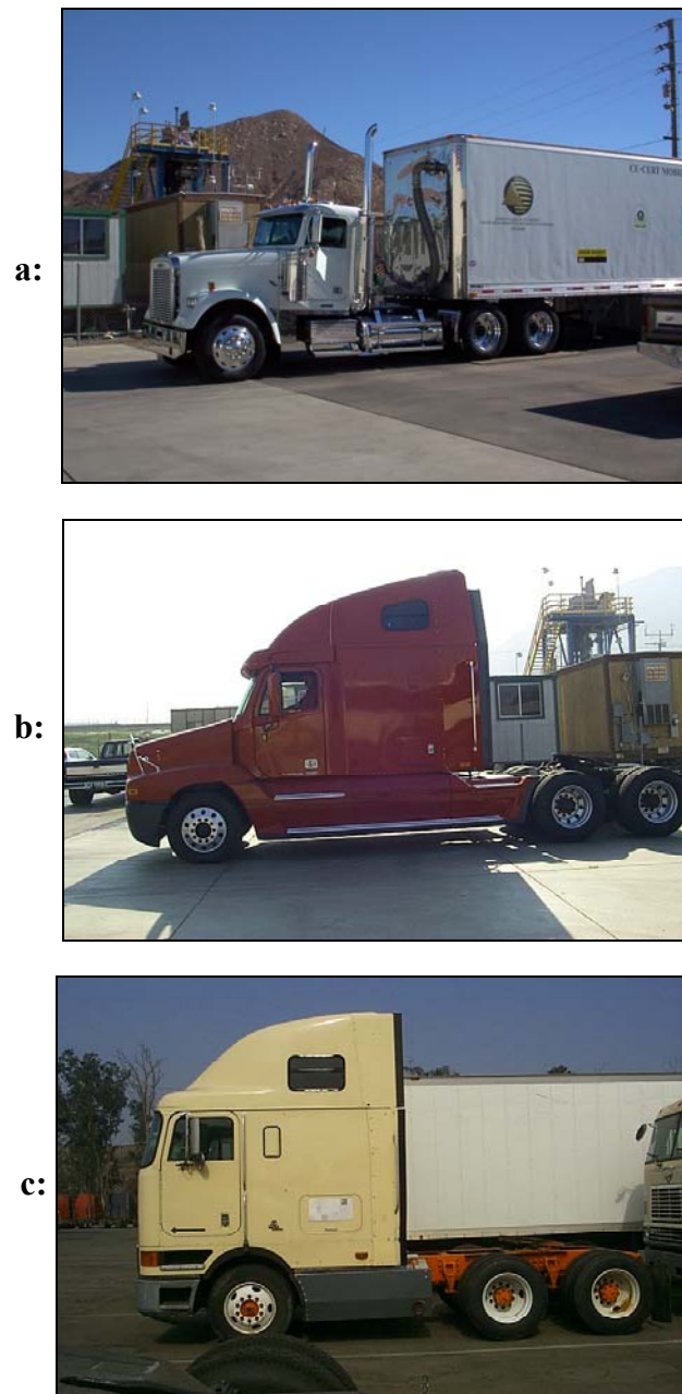
Figure 4.3. Example HDD truck shapes: a) Conventional Non-Sleeper Cab, b) Conventional Raised Roof Sleeper Cab, and c) Cab Over Engine Raised Roof Sleeper Cab.
