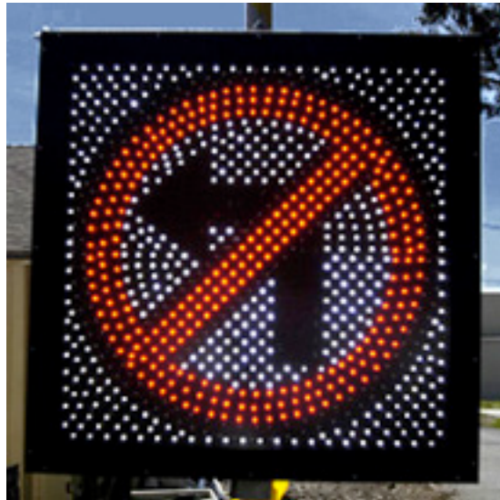
Figure 5. Left Turn Prohibited Sign Adapted to Active DII
