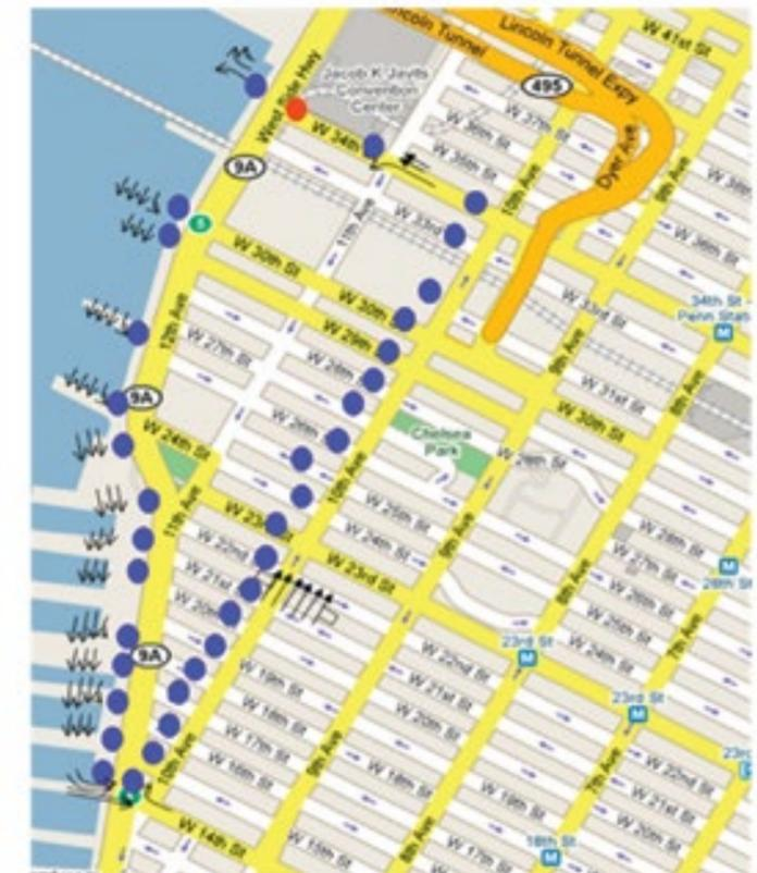
Figure 2 Map of NYC arterial route used for each NYC road test and the ITS World Congress demonstration. The red dot indicates the traffic signal nearest to the Javits Convention Center; the arrows show how many lanes and the blue dots are traffic signals.
