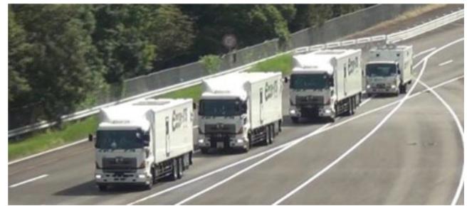
Fig. 6. The Energy ITS automated platoon of 3 heavy trucks and a light truck.
