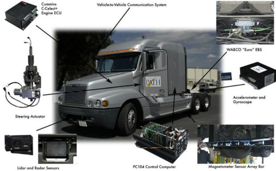
Fig. 11. Freightliner century truck tractor with PATH modifications for automation.
